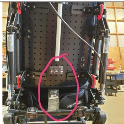
Back support serial number and size. These can also be found underneath the foam pad on the inside of the backrest shell.
